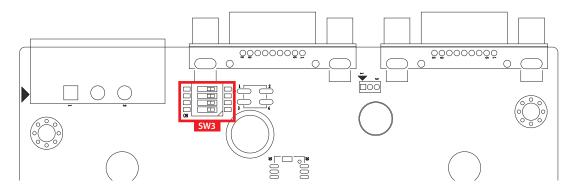
The EAC-4000 provides 16 different power on/off delay modes, which are adjustable via the SW3 switch. The default DIP switch setting is 0 in ATX power mode.
