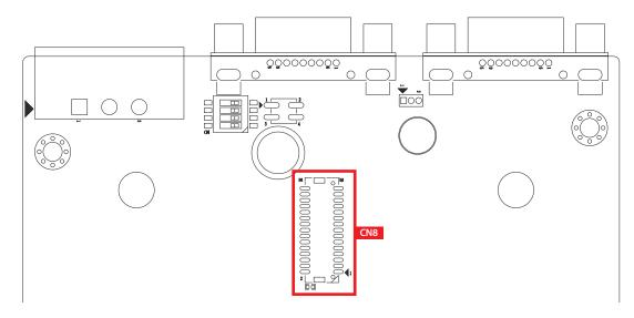
The CN8 connector provides debug UART, I2C, 4-wire UART, SPI, 7-bit GPIO, CAN bus, and ignition remote control functions. All signals operate at a 3.3V voltage level.
