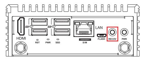
To enter Force Recovery Mode, press and hold the Recovery button.
