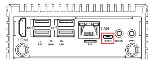
The EAC-4000 USB Recovery Mode provides an alternative boot device (USB). In this mode, the system is connected to a host computer and boots via USB. This mode is used when a new image needs to be flashed. USB0 must be available to function as the USB device for USB Recovery Mode.
