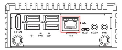
There is an 8-pin RJ-45 jack on the front panel of the EAC-4000 series, supporting 10/100/1000Mbps Ethernet connections. It supports 1000BASE-T gigabit data signals over standard Ethernet Cat 5 or Cat 6 cables.
