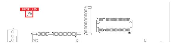
The MPCIE1\_LED is used to indicate the status of WAN, WWAN, and WPAN on the mini PCIe card.
