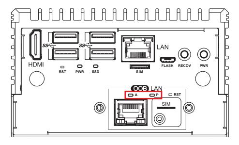
The LED indicator can instantly judge the power status of OOB Enabler and the connection status of OOB Enabler and Allxon Portal. If both LEDs are on, it means OOB Enabler is running and the connection to Allxon Cloud is stable.
