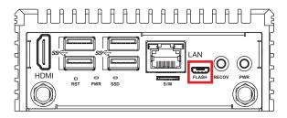
**Step 3:** Press and hold the "Recov" button on the EAC-4000.
