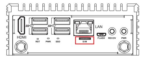
The external Nano SIM card enables wireless communication for the system when used with a mini PCIe 4G card.
