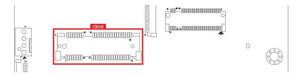
The EAC-4000 includes a Mini PCIe slot that supports PCIe signals.
