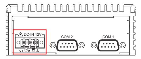
The EAC-4000 supports 12V DC power input via a terminal block.
