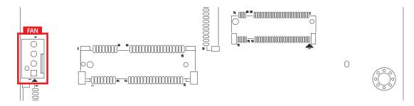
The FAN header supports additional thermal requirements.
