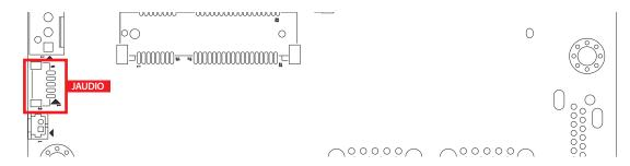
The connector is connected using an audio jack cable for line-out and mic-in applications.
