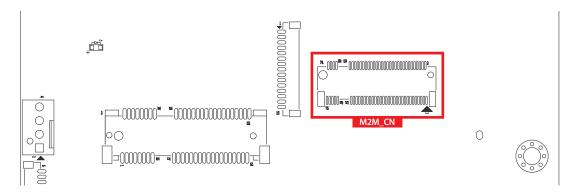
The M.2 Key M connector is suitable for applications that use host interfaces supporting PCle Gen 4 x4. It can accommodate an NVMe module card of the 2242 type.
