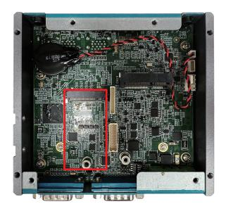
**Step 1** Install M.2 into the M.2 slot.
