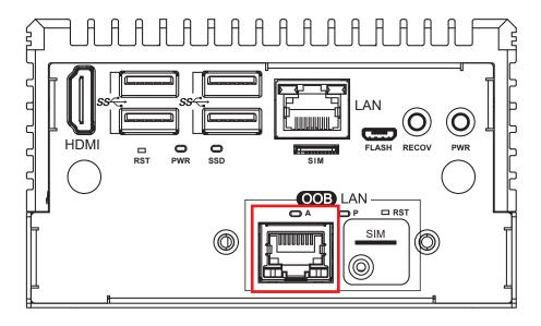
There are 8-pin RJ-45 port supporting 10/100 Mbps Ethernet connections in the OOB-100.
