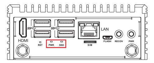
The PWR LED lights up when the system is powered on and ready. The SSD LED indicates storage activity.
