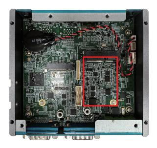
Step 1 Install Mini PCIe card into the Mini PCIe slot.
