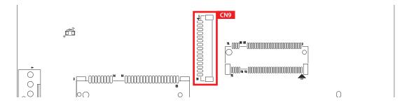
The connector is linked to the OOB daughter board, which enables remote control of system functions (such as power on, reset, or monitoring).
