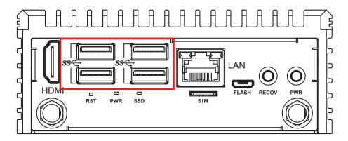
There are four USB 3.1 connectors available on the EAC-4000, supporting data transfer rates of up to 5 Gbps. They are also compliant with the requirements for SuperSpeed (SS), High Speed (HS), Full Speed (FS), and Low Speed (LS).
