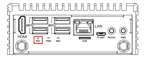
If the system encountered an error or becomes unresponsive, press the Reset button to restart the system. The operating system will then reboot.
