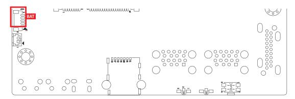
The BAT connector is connected to a CR2032 battery with a cable to supply power to the RTC IC. If the battery is disconnected, the RTC function will not work, and the operating system time will be incorrect.
