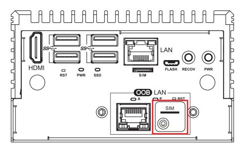
There are external Nano SIM card are assigned for mini PCIe slot respectively offer wireless communication capability to the system.
