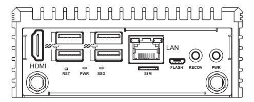
In the Vecow EAC-4000 series, most of the I/O connectors are located on the front panel. General connections to computer devices, such as HDMI, USB 3.0, LAN (RJ-45), flash port (Micro USB), recovery button, power button, reset button, SIM slot, and power and HDD LED indicators, are all placed on the front panel.
