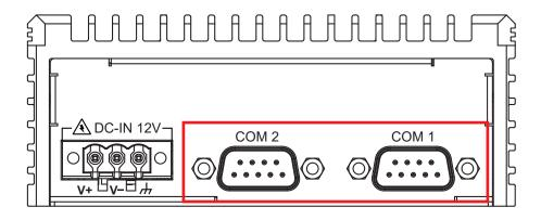
COM1 and COM2 can be configured for RS-232, RS-422, or RS-485 communication with automatic flow control. By default, COM1 and COM2 are set to RS-232 mode. To use RS-422 or RS-485, you must configure the ports through GPIO.
