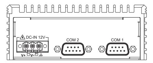
In the Vecow EAC-4000 Series, most of the I/O connectors are located on the front panel. The rear panel has only three I/O connectors, including the power terminal block and the COM ports.
